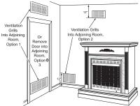
Figure 4 - Ventilation Air from Inside Building
